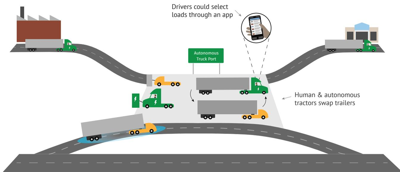
the freight to an ATP, where an autonomous tractor would take over, for instance. Since there would be a large volume of tractors and trailers continually moving through the same facilities, in theory there would be little reason that a particular autonomous tractor could not go to many or nearly all other ATPs. Tractors and trailers could be mated based on timing of their arrival to the ATP.
