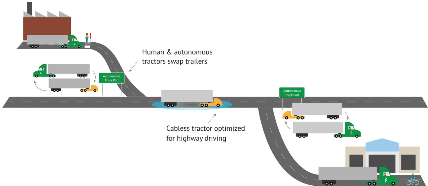
outbound trailer. That worker potentially could also ensure that the autonomous truck is safe to drive, fueled, etc. The autonomous truck would then drive the interstate portion of the freight's trip, while the human driver could take an inbound trailer from the ATP to final delivery in the local area.
